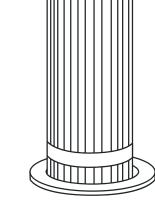
Insert Multifit cartridge in tube sheet, is easily secured by pressing it down by hand
