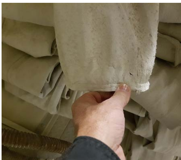
Holes in the bottom of a filter bag.
